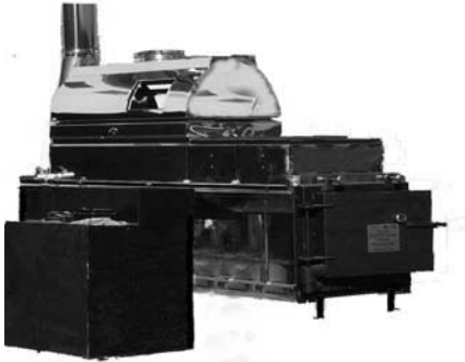
Wood pellet evaporator
